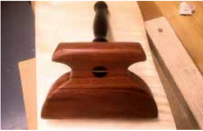
Telephone shaped veneer hammer with African blackwood handle
